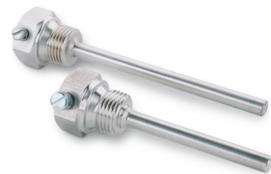
Example: Stainless steel sleeve for temperature sensor with installation length 85 mm and 120 mm with side clamping screw
