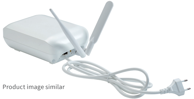
Gateway with integrated power supply unit and external antennas
